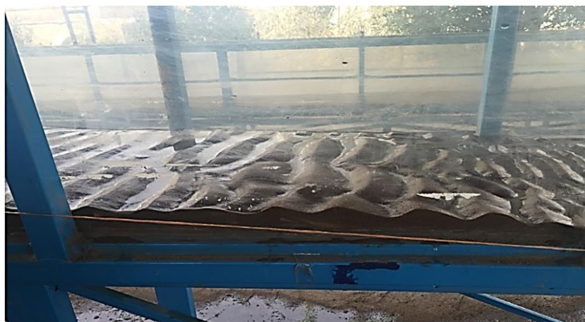
Fig. 6 Deformed state of the simulated beach after the end of the test period.
