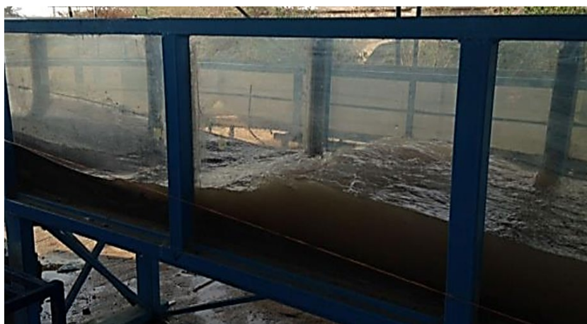
Fig. 5 The mode of wave interaction with the bed and the type of wave breaking on the shore slope during the experiment.
