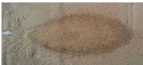
Fig. 2 A typical scour hole for test 30-10-3
