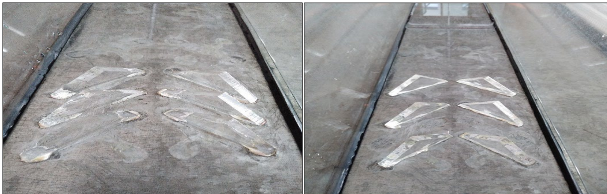
Fig. 1 Examples of the arrangement of equilateral triangle blocks in the trapezoidal channel of the present study
