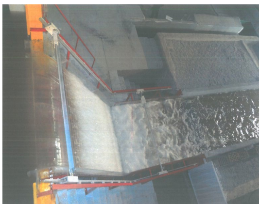
Fig. 5 Flowing over the stepped rapids and the stilling basin
