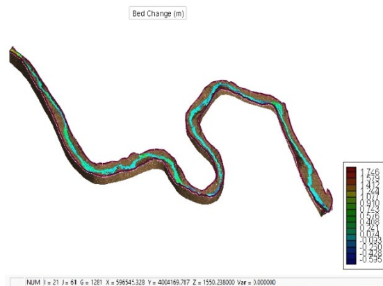
Fig. 9 An example of bed changes in an area of the sub-branch of the Khan River
