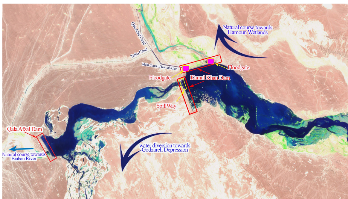
Fig. 4 Schematic of Kamal-Khan dam and its its infrastructures (Mamasani, et al., Forthcoming)
